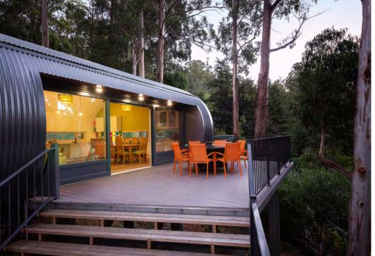
Inspired by the shape of a fallen log on Allan and Ann's Dandenong Ranges property, the house's curves are clad in corrugated iron for its flexibility and BAL compliance. As an added bonus, falling leaves and branches simply slide off, a plus in this bushfire-prone setting.
